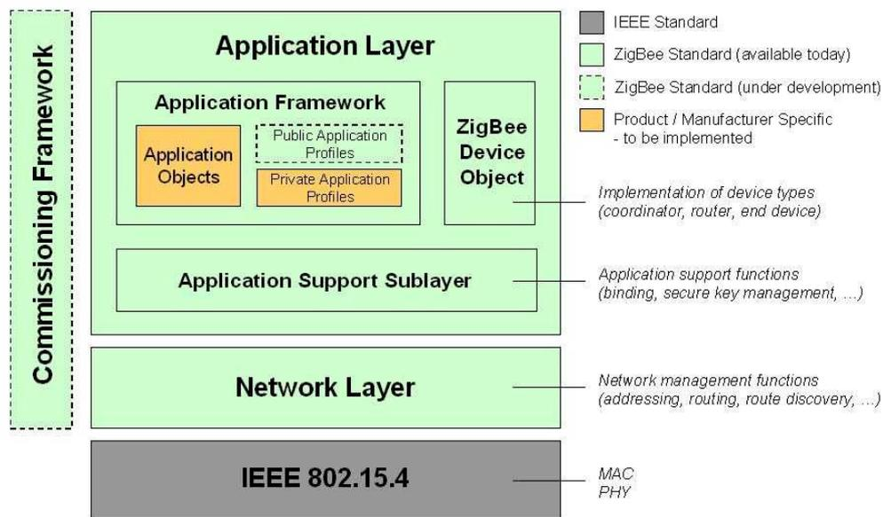
Figure 1 - ZigBee Protocol Stack
